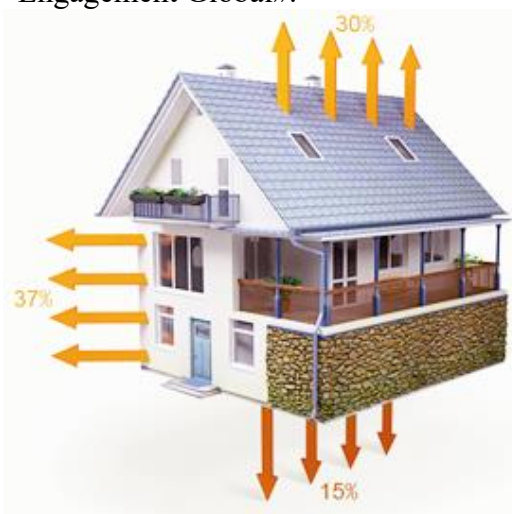
Fig. 1. Estimated heat loss in the building
