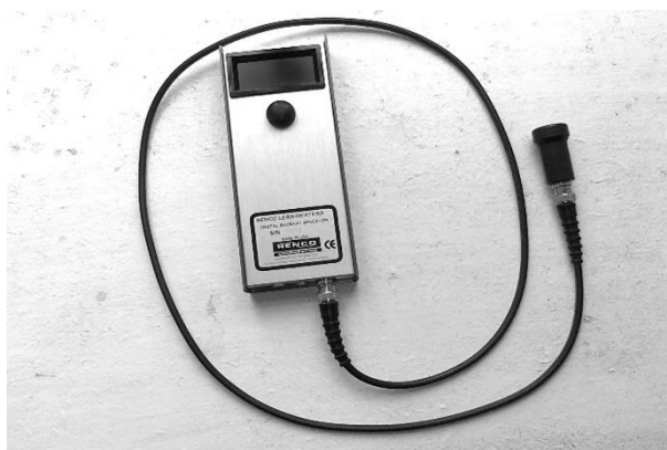
Fig. 1. Device for measuring the thickness of lard in pigs RENKO CE (RENKO LEAN MEATER DIGITAL BACKFAT IDIC, S/N 46080)
